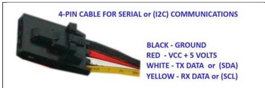
This connector can go to external Bricks or other devices that have more complex Communications Protocols to work with Arduino. Examples are GPS receivers, Ethernet interfaces, and other complex devices. These are 4-pin connectors.
